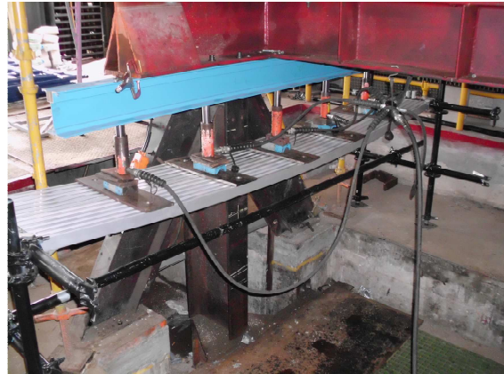
Failure by deflection
