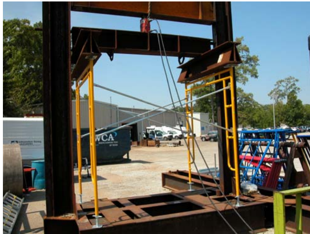
Set up for compressive load testing. Set #2
