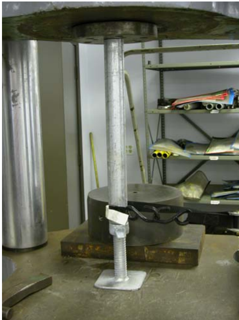
Compressive load test configuration.
