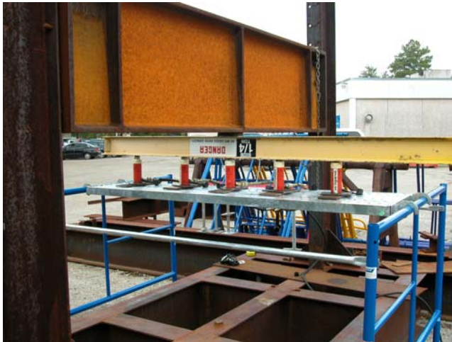
Uniform load test configuration
